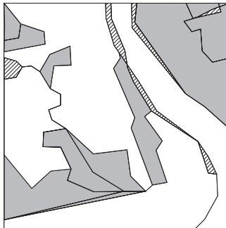
Figure 15: Classification map using k_o -threshold of 0.1, showing fused extents where t \in T_1 \cup T_2 (white shading), t \in \text{Im}(g_1 \otimes g_2) \setminus T_1 \cup T_2 (gray shading), or where extent is unclassifiable (hatched shading)
