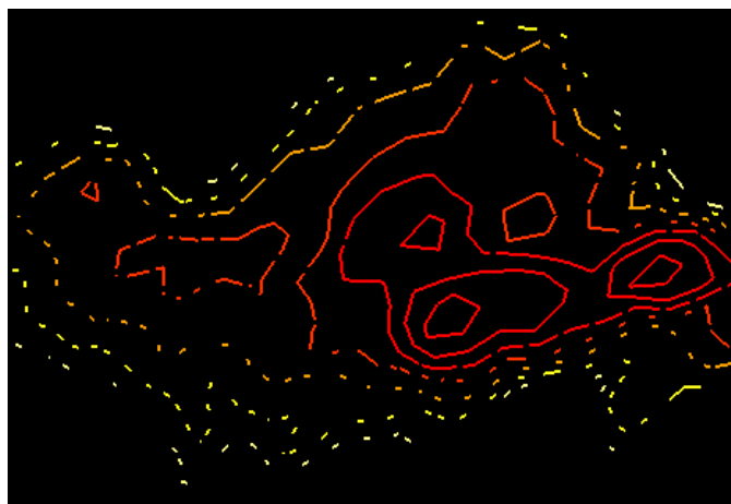
Figure 2: Spatial uncertainty is encoded as gaps in contour lines. The more uncertain, the larger the gaps. The contour lines themselves are for some other variable such as temperature, humidity, etc.
